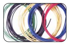
Series PEFR, Flame Resistant - Excellent stress crack resistance. Preferred product for pneumatic control applications in the HVAC and energy conservation industry. Working pressure up to 185 psi. -85°F to 150°F. Sizes 5/32" - 1/2" O.D. Meets UL94V-2 flame classification. Black.
